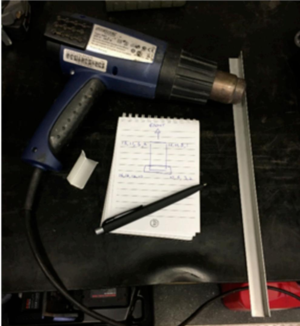
Use the [HD2 Video Preview](#) feature, either on a mobile device or a laptop, and then move the hot object in front of a sensor at chosen spots on across the tyre surface. The Heat Block elements in the calibration scene will react as you move the hot object in front of each sensor.
