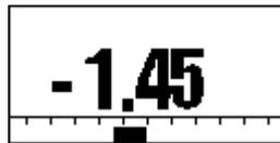
Once a valid reference lap has been created or loaded, the VBOX Mini will begin predicting. The prediction is shown in text and graph format which is a graphical representation of the amount of time gained or lost around the lap.
