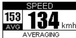
This screen can be used to average a vehicle's speed between two locations, allowing calibration of a speedometer or other velocity-measuring such equipment. The start point can be either of the following:
