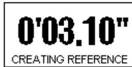
If you do not have a reference lap file, you will have to wait until a full lap of the circuit has been completed. This screen will be displayed while the drift box is creating a reference lap.
