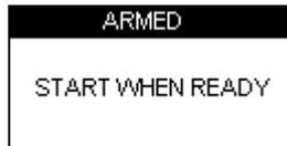
4. When this screen appears, the unit is ready and lap timing will commence as soon as the vehicle starts moving. Timing will end when the vehicle crosses the start / finish line.
