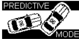
Predictive mode enables you to graphically view your predicted lap time. Predictive lap timing works by saving your position around a circuit, every second. If the current lap is the fastest so far, then this positional data is saved as a reference.
