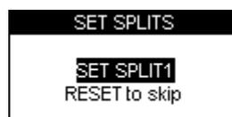
5. To set the first Split, press **OK** when the vehicle passes this point, or press **RESET** to skip setting of this line. Repeat this for each of the split lines.
