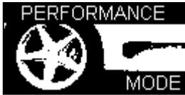
The Performance mode is used to measure the acceleration and braking performance of a vehicle. Press the **MODE** button to scroll to the Performance Mode screen. This mode is divided into thirteen screens, each of which displays different performance data. Navigate between these screens by using the ▲▼ buttons. Each screen will automatically display the results as they happen, for example if you drive from 0 mph to 60 mph then the 0-60 section will show the time taken.
