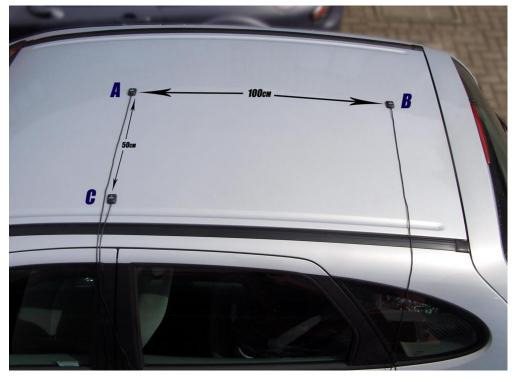
The picture to the right shows a typical 3-antenna placement for the measurement of Body Slip Angle, Pitch and Roll angle. Antenna A the primary antenna is placed in the centre of the roof. Antenna B is placed behind Antenna A, allowing True heading, Slip angle and Pitch Angle to be measured. Antenna C is placed to the side of Antenna A allowing the measurement of Roll angle.
