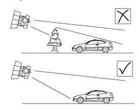
NOTE: VB20SL3 can struggle with maintaining an RTK lock required for Slip, Pitch and Roll measurement if the antennas are placed too close to Roof Bars. If a poor mounting position cannot be avoided then use Ground plane antennas, RLVBACS065.
